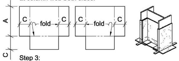
Cut & apply target patch over finger flashing with 2" overlap.
