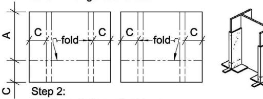
Cut & apply finger flashings at column web both sides.
