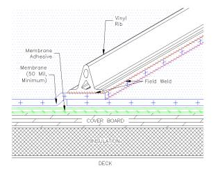
Refer to Detail Drawings VR1001, VR1005, VR1010, VR1015 and the Vinyl Rib Roofing System Specification for installation instructions.
