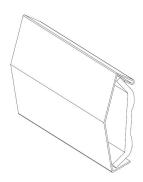
1.75-inch (44 mm) wide Metal Fascia System (Install per detail drawing 3500 or FA3500)
