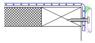
1.75-inch (44 mm) wide Fascia System (Install per detail drawing 3030 or FA3030)
