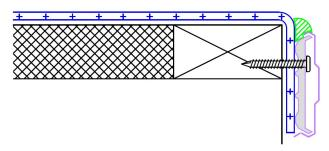
4-inch (102 mm) wide Fascia System (Install per detail drawing 3040 or FA3040)
