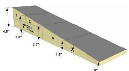
Figure 2. Duro-Guard ISO II Taper
