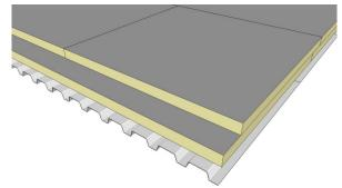
Figure 1. Duro-Guard ISO II Flat On Steel Deck
