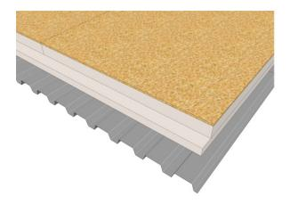
Figure 1. Duro-Guard EPS Nail Base
