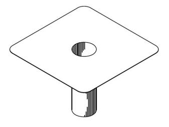
Drain Boot (Install per detail drawing 2020)
