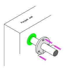
Conduit/Escutcheon Washer (Install per Detail Drawing 4100)
