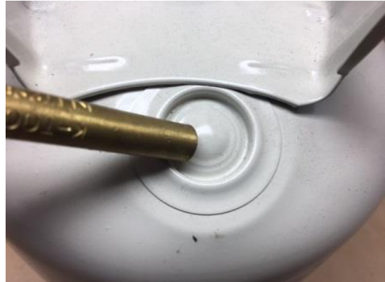
Location of rupture disk
