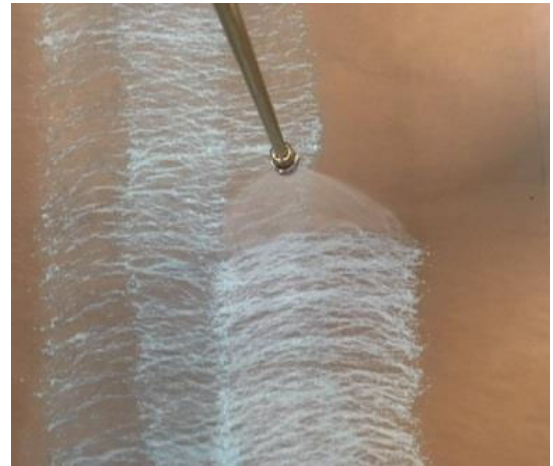
50% overlap spray pattern (Blue color is used for photo representation only.)
