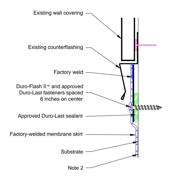
Note 1: Minimum termination height for parapet wall flashing is 8 inches above finished deck. Refer to Detail Drawing 6020.
