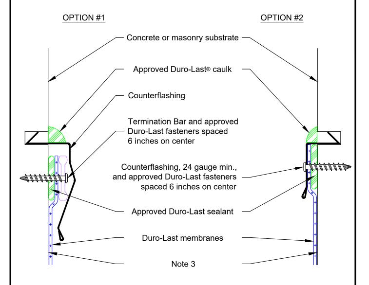
Note 1: This detail is only applicable with concrete or masonry walls.
