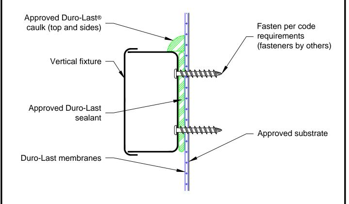
Note: Bottom of vertical fixture shall be a minimum of 8 inches above the finished roof deck.
