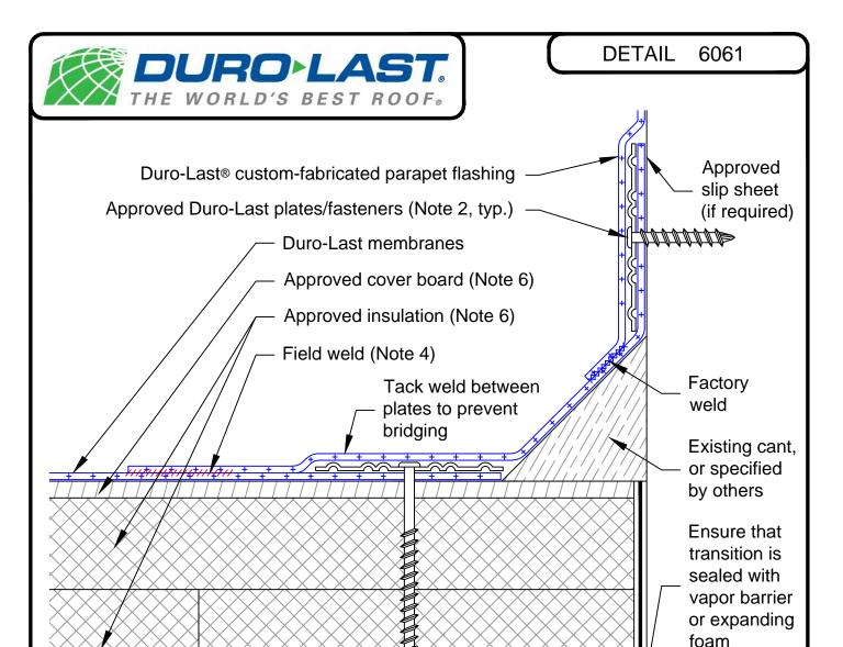
Note 1: Minimum termination height for parapet wall flashing is 8 inches above finished deck. Refer to Detail Drawing 6020.
