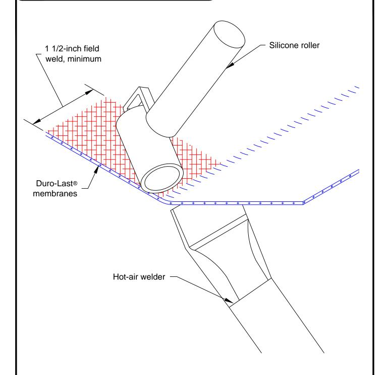
Note: After any field seam is completed, it must be probed to ensure that a secure weld has been made.
