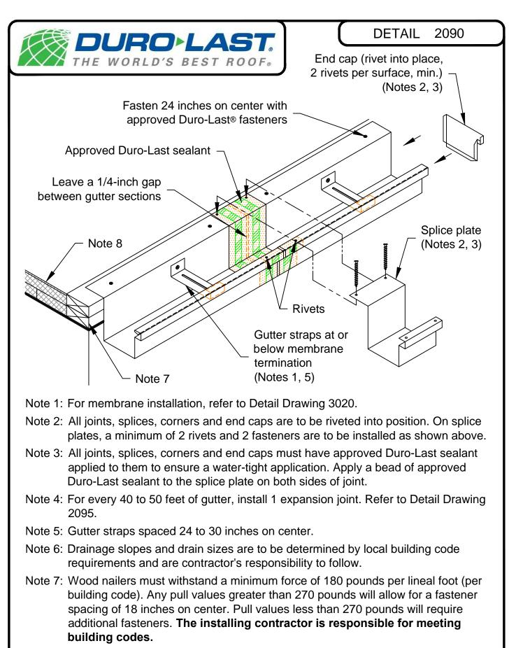
Note 8: Refer to specifications for vapor barrier, insulation and cover board requirements.
